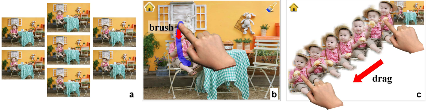
Figure 1. The brush-and-drag interface. (a) A given group of similar photos. (b) We use a natural brush gesture with our finger(s) to mark an area/object of interest in one of these photos. Our tailored segmentation engine quickly segments the corresponding image elements in the photo group. (c) We can then drag the segmented image elements to spread them out for better examination. This user-centric design allows the user to decide the size and the area of interest. It also maintains the overall photo context while enabling the user to focus on the selected area of interest for comparison and photo triaging (focus+context). Note that the normally black background of the tablet display was changed to white for printing purposes.
