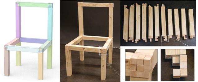
Fig. 20. Interlocking  $1.0m \times 0.5m \times 0.5m$  Frame Chair. The voxel joints are fabricated by gluing wooden cubes in the spatial arrangement computed by our algorithm. When attached to the corresponding wooden pillars, all pillars can be connected into a steady interlocking assembly.
