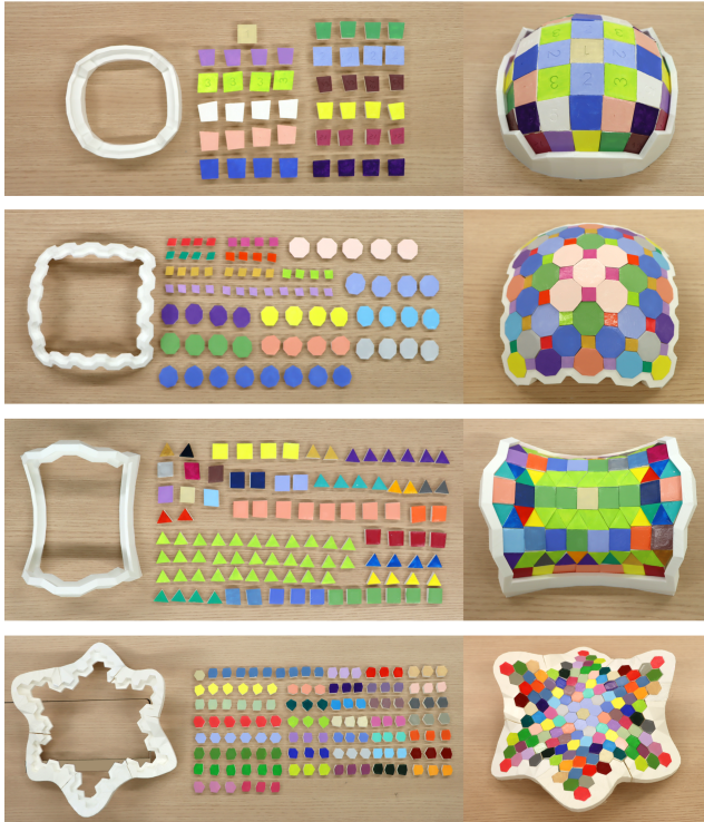
Fig. 17. 3D printed shell elements and assembled shell structures. Shell elements in the same class are painted with the same color.
