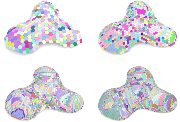
Fig. 16. Reusability of shell elements improves when there are more shell elements used for approximating an input smooth surface; see also statistics in Table 1.
