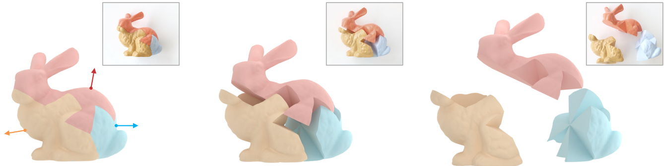
Fig. 1. We propose a computational approach for designing coordinate-motion assemblies, which can be disassembled only by using a coordinated motion of component parts specified by users. We demonstrate this with a three-piece BUNNY assembly. The columns display the initial, intermediate, and fully disassembled configurations, with the physical prototype (top) matching the virtual design (bottom). Colored arrows indicate the translational directions along which the parts must move simultaneously to reach the next configuration.
