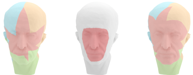
Fig. 14. Users can select a protected region (middle) to preserve salient features during part decomposition. Compared to the result without user guidance (left), our guided design better preserves the human facial features (right).
