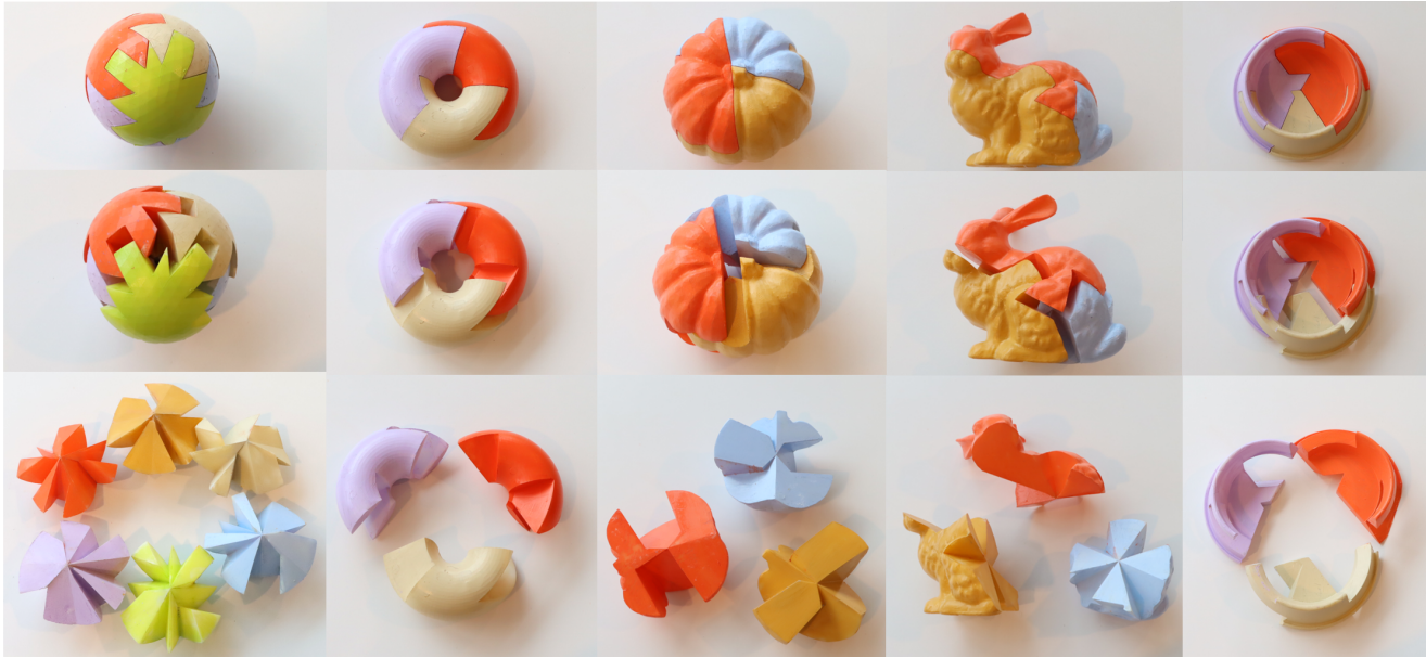
Fig. 15. The disassembly sequence of our 3D-printed results. The fabricated prototypes confirm that our designs realize the intended disassembly via unique coordinate motion.
