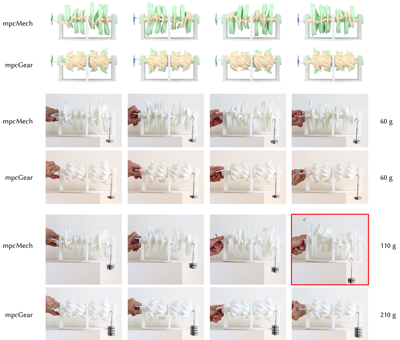
Fig. 12. Comparison of load-bearing performance between mpcMech and mpcGear through a physical experiment. (Rows 1-2) Four key poses of mpcMech_3R and mpcGear_3R generating the same motion, where the leftmost column shows the first key pose. (Rows 3-4) mpcMech_3R and mpcGear_3R both carrying a 60g load. (Rows 5-6) mpcMech_3R carrying a 110g load and mpcGear_3R carrying a 210g load.
