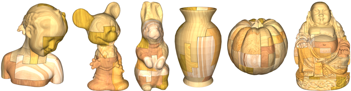
Figure 9: Various 3D interlocking models created by our approach: 8-parts BIMBA, 10-parts MICKEY, 16-parts RABBIT, 10-parts VASE, 16-parts PUMPKIN, and 20-parts BUDDHA (from left to right).
