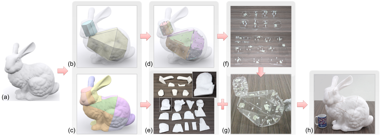
Figure 2: Overview. (a) input model; (b&c) optimized results: coarse polyhedrons (internal bases) and fine 3D-printed parts (external shell); (d) interlocked laser-cut assemblies; (e) 3D-printed parts; (f) laser-cut parts; (g) assembled laser-cut bases; and (h) final assembled object.
