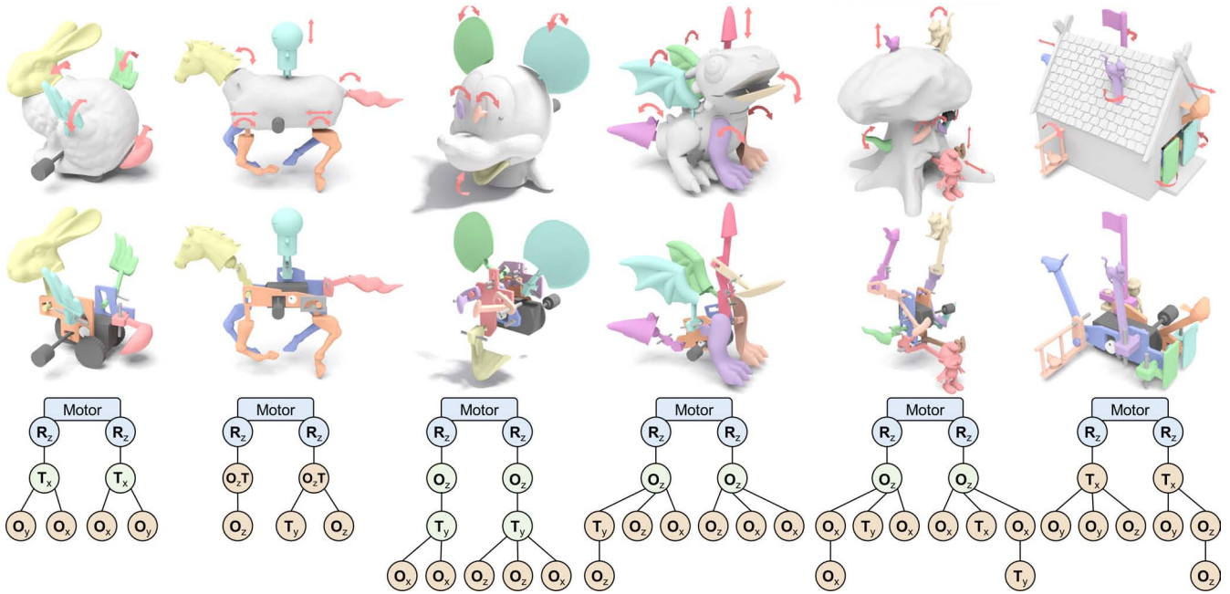
Fig. 14. Some of the wind-up toys produced from our system; from left to right: BUNNY, HORSE, MICKEY, DRAGON, TREE, and HOUSE. From top to bottom: input models and prescribed toy part motions, the optimized wind-up mechanisms, and the associated motion transfer trees, where we color the nodes connected to the external toy parts in orange.
