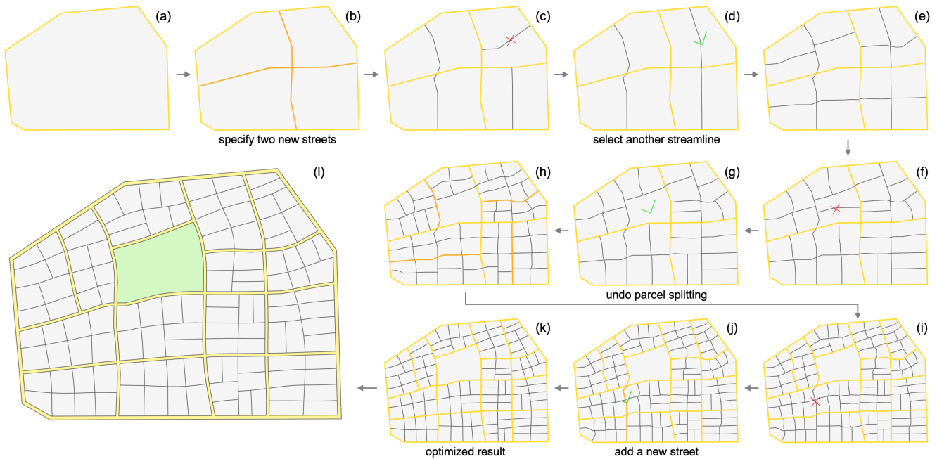
Figure 15: Users are allowed to locally control the generation process of parcels and streets at each hierarchical level, including (b) specifying two new streets (in orange), (d) choosing another streamline for generating new parcels, (g) undoing partitioning on a parcel (for using it as a park), and (j) editing the generated street network by adding a new street. The resulting urban layout is shown in (l), where the green parcel is the park.
