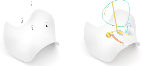
Fig. 7. (Left) User inputs are a reference surface S , a target 3D path represented by a sequence of 3D points \{\mathbf{p}_j\} (in purple color), and a desired mobility type (transmobility in this example). (Right) Our approach designs a conformable mechanism that conforms to the reference surface S and generates a 3D path (in green color) that approximates the target one.
